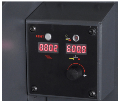
Easy setting of the motorised back-gauge, and cut-counter from the front of the shear.
